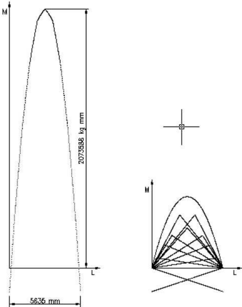
左图为底梁弯矩图，右图为各分力在底梁上产品的弯矩图。Bottom beam bending moment diagram is on left picture, Each component on the bottom of beam bending moment diagram of the product is on right picture.
